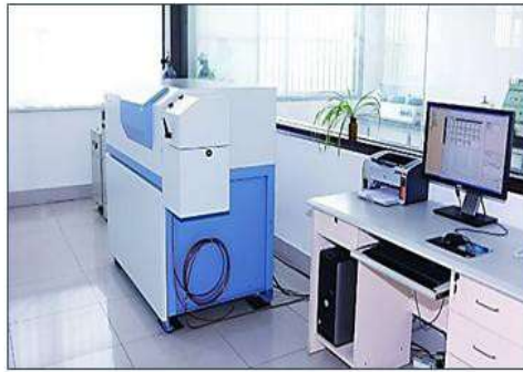
光谱仪Spark Direct-reading Spectrometer (Switzerland) (29个通道24个元素)
